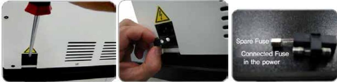
2. If you find the fuse broken or damaged, replace it by the new spare one stored in the fuse case and check out if the power can be turned on.
